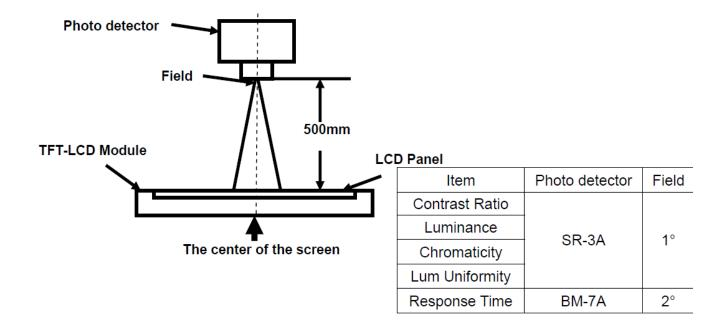
Note 2: Definition of viewing angle range and measurement system. viewing angle is measured at the center point of the LCD by CONOSCOPE(ergo-80).
